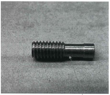
Closed center components open center plug can be found below LS plug on all inlets
